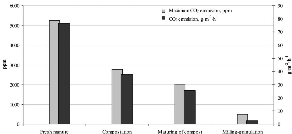
**Fig.2. Measured carbon dioxide (CO<sub>2</sub>) emissions from technological operations of milled compost and granule production**
